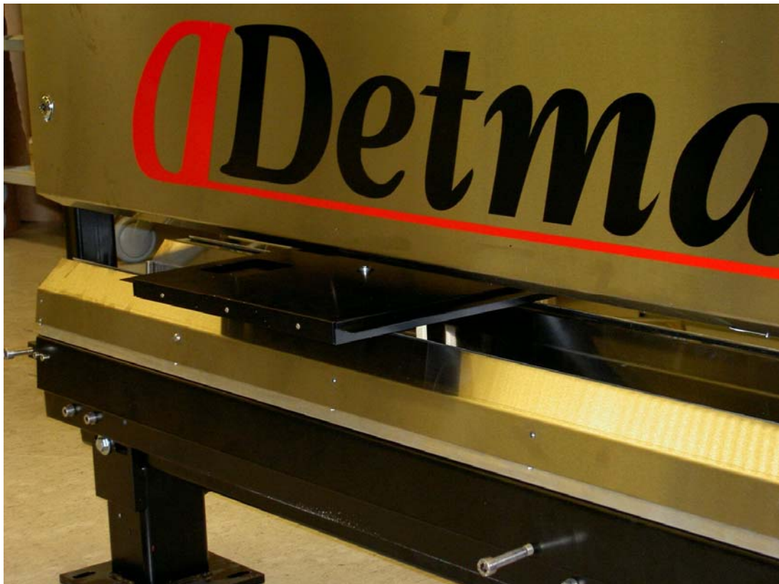
Box for rotating verification disc including hole samples.
